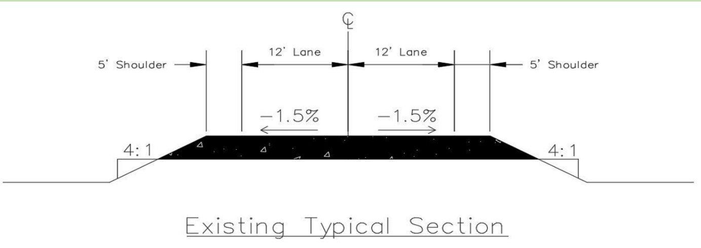
Figure 16: Existing Typical Cross Section [7]
